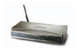
The PLANET WRT-414 is an 802.11g compliant Wireless Broadband Router that is designed for sharing Internet connection to all LAN and WLAN clients at the same time. It supports 64/128-bit WEP (Wired Equivalent Privacy), WPA-PSK, WPA, WPA2 Encryption and MAC/IP filter access control for securing wireless network connection. Not only AP mode, but also AP Client, Bridge and WDS mode are supported. The WRT-414 provides more flexibility for users when they establish wireless network.
