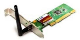
Complying with the newly approved 802.11g standard, WL-8316 provides a faster wireless connection for laptop users who want to access network resources. The gadget delivers data at speeds up to 54Mbps, 5 times data rate than 802.11b.
