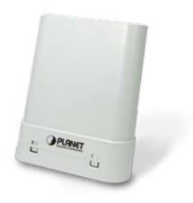
PLANET Technology provides an outdoor wireless solution with higher coverage and stronger functions- the wireless LAN outdoor CPE AP/Router, WAP-6200. It is compatible with IEEE 802.11b/g, offering the data rate up to 54 Mbps. With the built-in 14dBi patch antenna and the default 200 mW transmit output power, the WAP-6200 is quite suitable for wireless LAN applications in widely open spaces.
