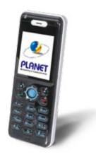
Based on years of VoIP manufacturing experiences, PLANET Technology introduces the 802.11b/g Functional Wi-Fi Phone, VIP-193, to offer a portable Wireless Voice over IP (WVoIP) solution. The VIP-193 is a cost-effective, easy-to-install and simple-to-use mobile phone that unleashes your voice communications free from wire.
