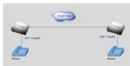
Peer-to-peer VoIP communication --- each site requires a PLANET analog telephone adapter
