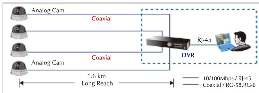
IP Cam quick expansion ↓ Reuse Coaxial Cable
