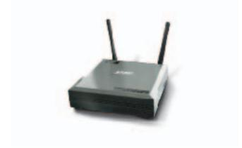
The MAP-2100 is designed with IEEE 802.11a/b/g standards and addressed on providing a high scale mesh network. All mesh nodes can operate at 2.4GHz for long range and better penetration, or at 5GHz to minimize the frequency interference. The detachable antennas design allows users to use proper antennas for various deploying requirements.
